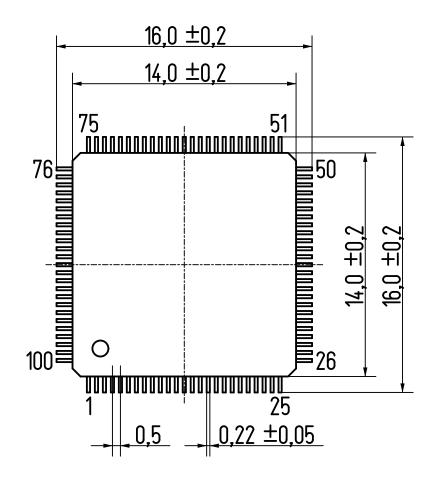
Package thickness: 1.4 mm ±0.05 mm All dimensions: mm
