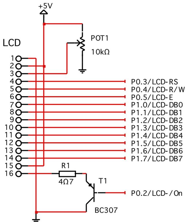
Pot1 is used to set the contrast of the LCD. T1 and R1 drive the power for the backlighting. This circuit is sufficient for displays which have a LED type backlighting.
