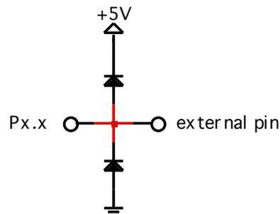
The diodes will short circuit any input voltages lower than 0V to ground and any higher than supply voltage to +5V.
