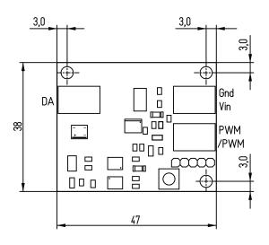
Dimensions in mm Height at thickest point: < 6.5 mm Tolerances: Outer contour: ±0.2mm
