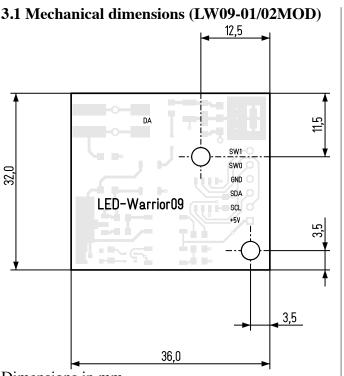
Dimensions in mm Height at thickest point:  $\leq 6.1$  mm Mounting holes: 3.1 mm Tolerances, outer contour:  $\pm 0.2$  mm
